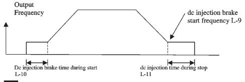
L-9: DC injection brake start frequency
