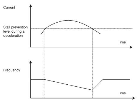
While running (no acceleration, no deceleration) if drive output current exceed this limit, drive begins decelerating (as per the set deceleration time) till current falls below this limit. When the current drops below the stall prevention limit, drive accelerates to set speed.
