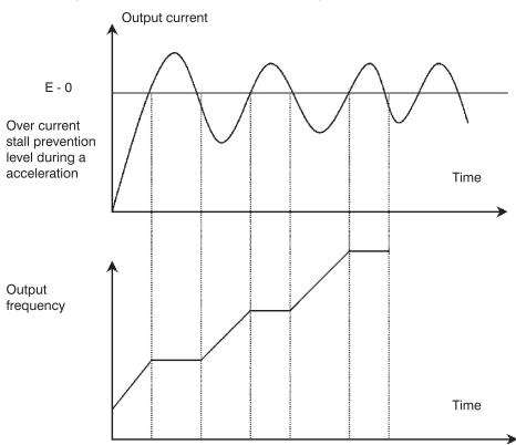
During acceleration if drive output current exceeds this limit, acceleration stops and drive continues to run at the same speed. Acceleration resumes when current falls below the stall prevention limit. Above value is a percentage of drive output current rating.
