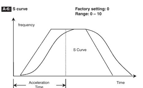
The S curve is for smooth acceleration and deceleration of the drive. If set to 0 it is deactivated. For a higher value, the speed time curve is no longer linear. With s curve the acceleration and deceleration times are higher than their set values.
